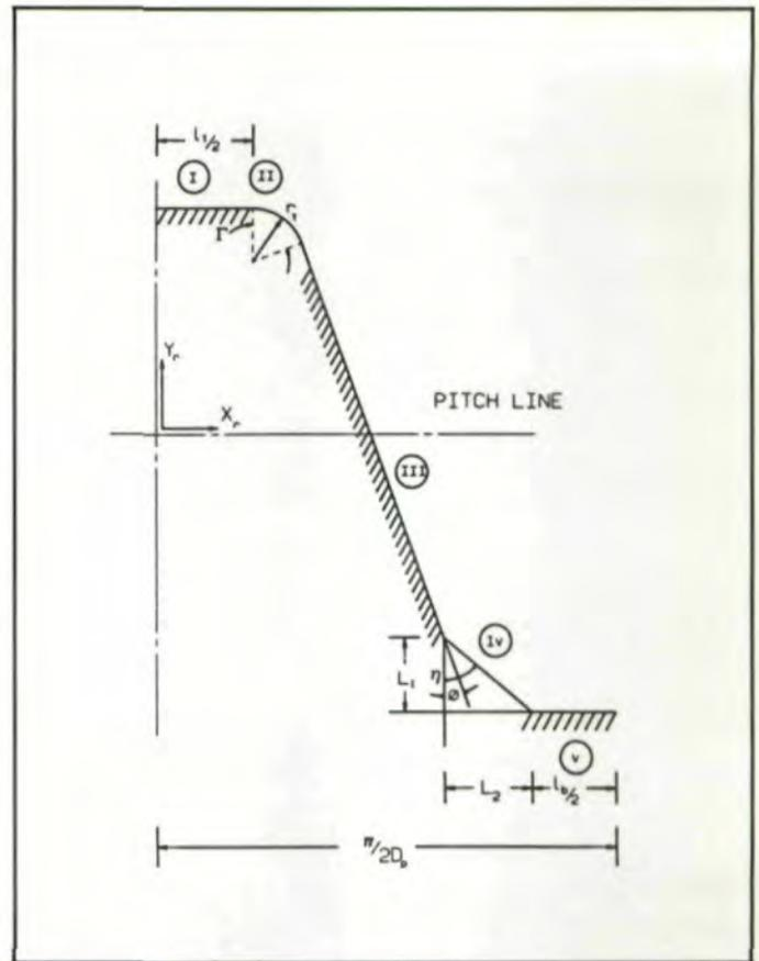
Fig. 8—Geometry of a hob with root chamfer.
