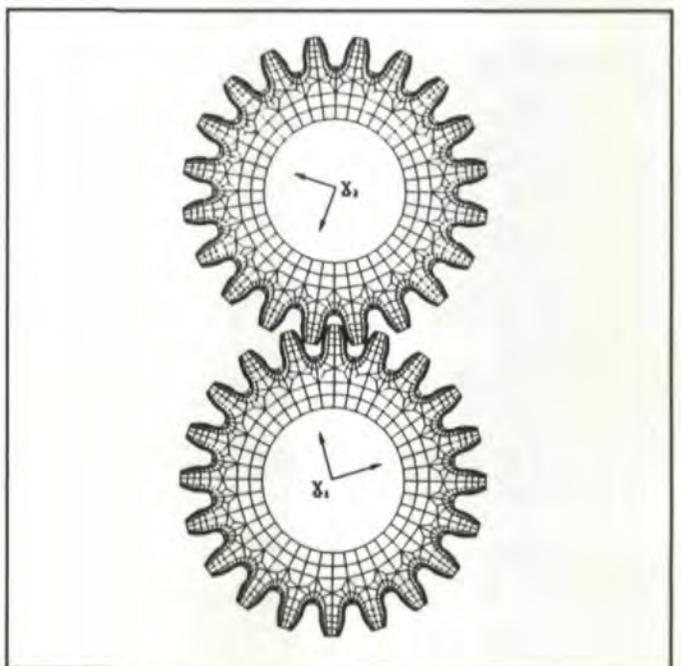
Fig. 19—Finite element model for contact analysis.
