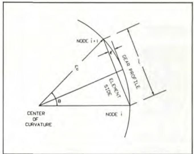
Fig. 17—Discretization error in the gear tooth profile.
