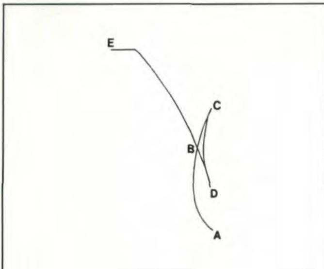
Fig. 4—Gear tooth profile generated when undercutting occurs.
