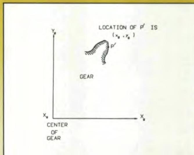
Fig. 2 – The gear and its attached coordinate system.
