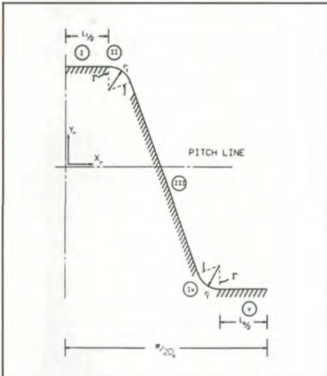
Fig. 6 - Geometry of an elementary rack.
