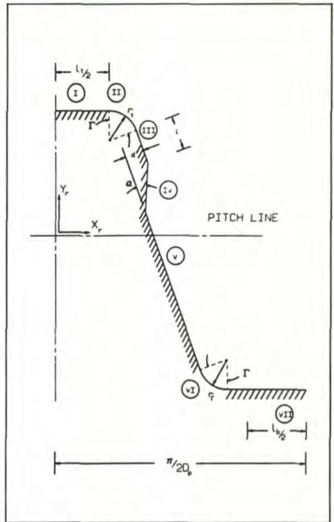
Fig. 7—Geometry of a rack with a protuberance.
