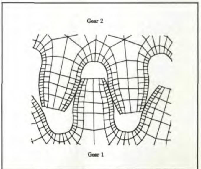
Fig. 18—Finite element model for contact analysis.
