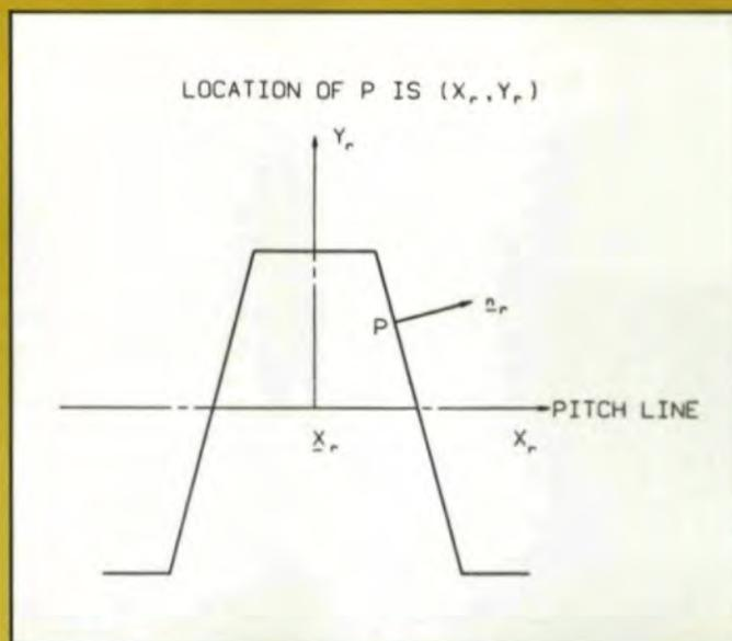
Fig. 1 – The rack and its attached coordinate system.
