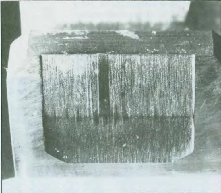
**Fig. 10 - General and destructive scuffing on a gear wheel. Note an important wear of the profile with the presence of radial rough irregular streaks. Also note a metal pull-off toward the tip of the tooth.**
