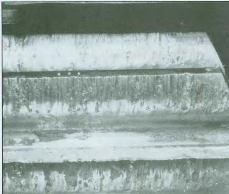
**Fig. 11 - Cold scuffing on the teeth of a winch wheel.**
