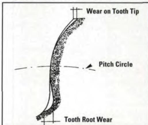
Fig. 1 - Distinctive aspect of distortion of gear tooth profile under wear action
