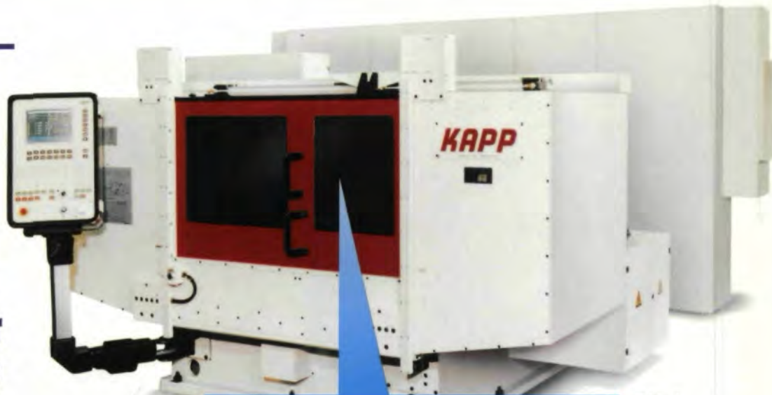
Critical gear tooth elements are measured by the Integrated Measurement System.
