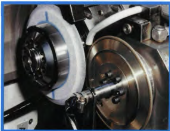
Information is fed back into the CNC for automatic correction by the dresser.
