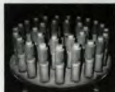
Fig. 2 — Parts as loaded for ion nitriding on the furnace hearth plate.
