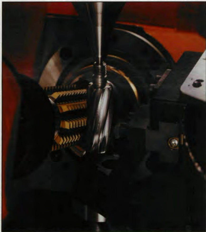
View of the pinion, hob and tailstock in the Liebherr LC 82. The workpiece load/unload mechanism built into the hobber, closely coordinated with workpiece clamping, reduced Ford's chip-to-chip time to about 4 seconds.
