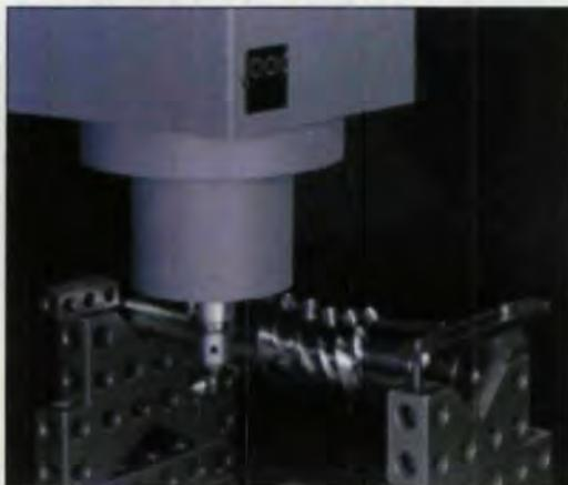
Right: Worm being inspected on a CMM. Courtesy of Brown & Sharpe.
