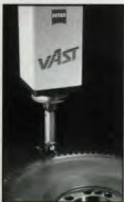
CMM inspecting a spur gear. Courtesy of Carl Zeiss, Inc.
