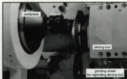
Fig. 6—The skiving tool can be reground in the machine. Source: Pfauter
