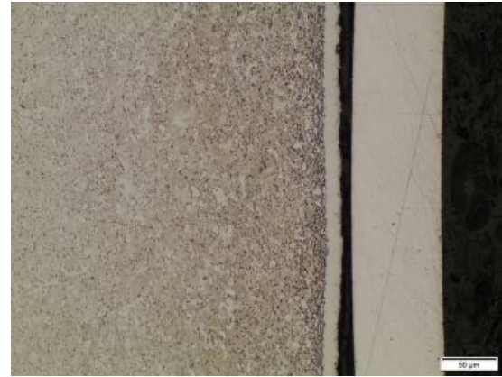
B. 200X mag. (White Layer = 13-18 microns HV = 500)
