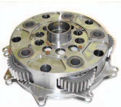
Figure 9—Second-stage carrier assembly.
