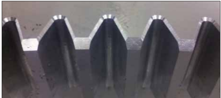
The Gear Chamfering Robot from Banyan Technologies is suitable to deburr, chamfer or radius the edges of slew bearing ring gears (courtesy of Banyan).
