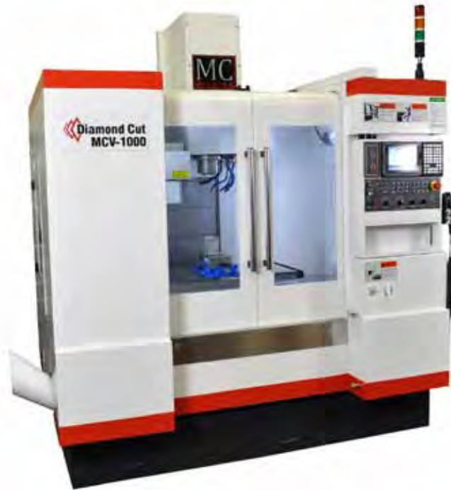
including fixtures, mold base, and secondary operations. The series comes with coolant-thru-spindle preparation and an M70 Mitsubishi controller. The machine can be equipped with a ZF gearbox to achieve four times the torque of a standard motor.
