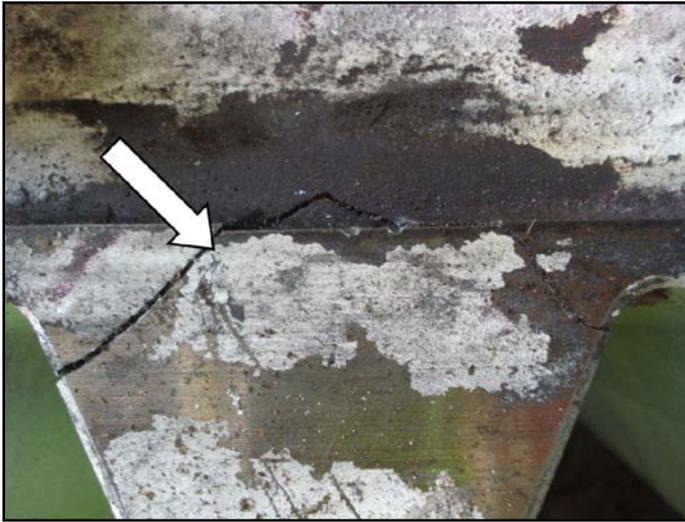
Figure 3 Tooth root crack due to misalignment.
