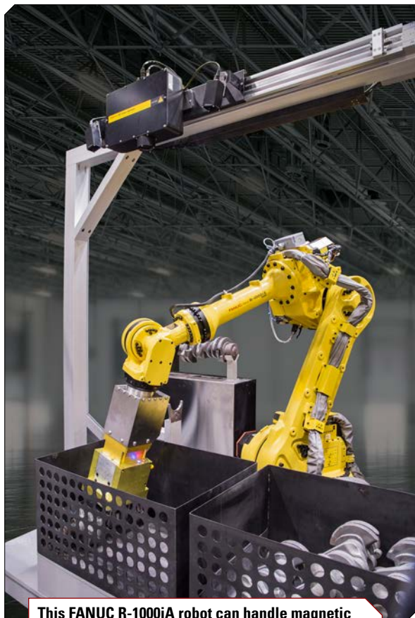
This FANUC R-1000iA robot can handle magnetic bin picking operations (courtesy of FANUC).
