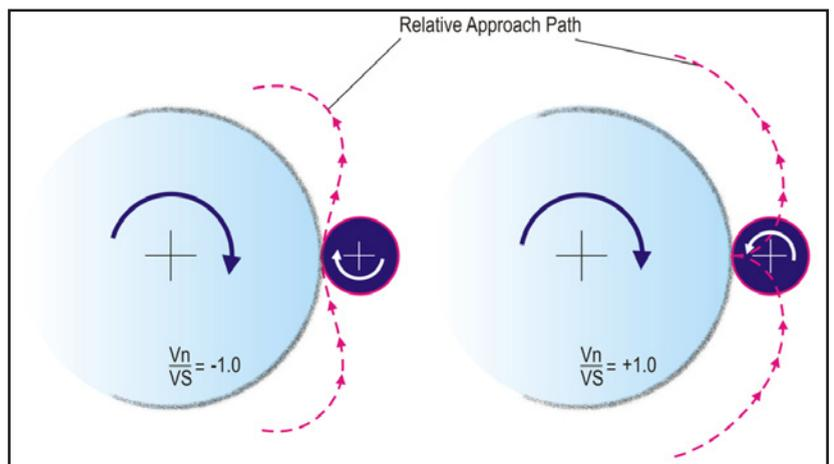
Figure 2 Pure shearing (left) and pure crushing (right).
