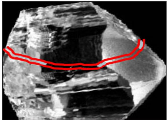
Figure 3 Principal appearance of a grain shear fracture.
