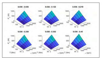
Figure 5—Predicted mechanical power loss for 0036 surface parings.
