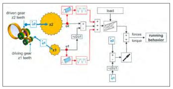
Figure 3—Influences on the running behavior of mating gears.
