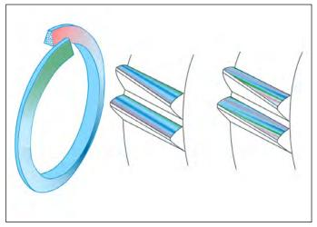
Figure 6—Flank surface modulation.
