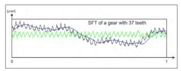
Figure 4—SFT with mesh transmission error.
