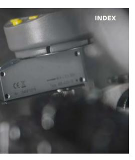
The CenterMaster system allows operators with no specialized knowledge or experience to set up a drill in two to three minutes. Additionally, it provides a repeatable accuracy of  $<5 \mu m$ .
