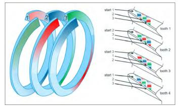
Figure 7—Flank surface modulation.
