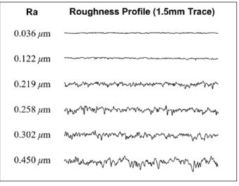
Figure 2—Magnified roughness profiles.
