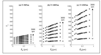
Figure 8—Predicted power loss vs. composite roughness.
