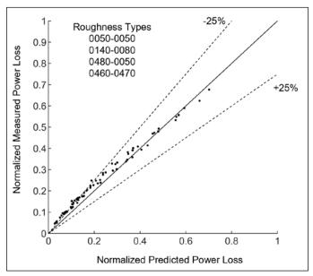
Figure 1—Model predicted power loss as compared to measured mechanical power loss. Adapted from Ref. 1.
