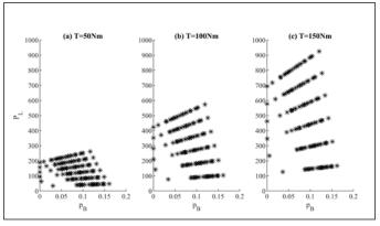
Figure 10—Predicted power loss vs. boundary area contact ratio.
