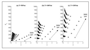
Figure 9—Predicted power loss vs. film parameter.
