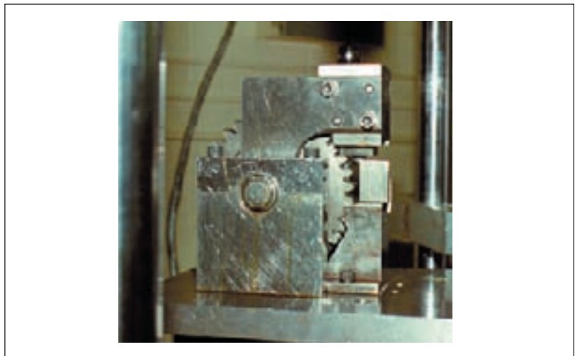
Figure 2—Gear Research Institute's standard STF specimen mounted in fixture.
