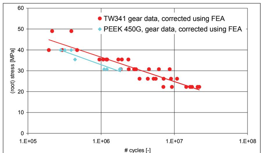
**Figure 8—Root stresses (corrected for tooth bending) versus number of load cycles for gear testing of Stanyl TW341 (red) and PEEK 450G (cyan) at  $140^\circ\text{C}$ .**
