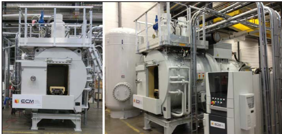
Figure 1 Multi-purpose vacuum furnace installed in Höganäs pilot plant.
