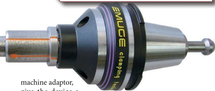
machine adaptor, give the device a quarter turn, and then hit a button on the machine controller, at which time the device is pulled back into the tapered spindle.
