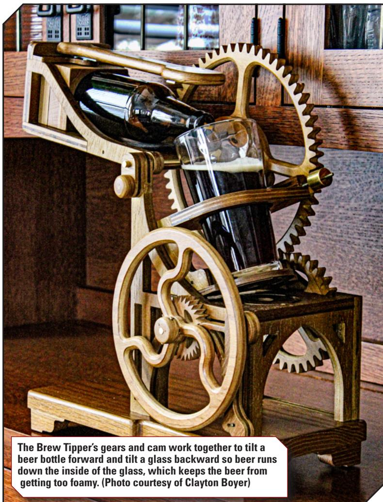
The Brew Tipper’s gears and cam work together to tilt a beer bottle forward and tilt a glass backward so beer runs down the inside of the glass, which keeps the beer from getting too foamy. (Photo courtesy of Clayton Boyer)
