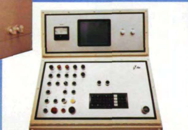
Operator's console has a grinding spindle load meter, a CRT screen and a keyboard for entering hob diameter, number of flutes, stock removal per rough and finish pass and number of passes, feed rate and right and left stroke limits. A CNC programmable controller is employed for sequence logic, feeding the grinding spindle slide, and positioning the hob spindle.
