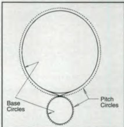
Fig. 2—Involute geared transmissions are ideally equivalent to crossed-axis belt drives.
