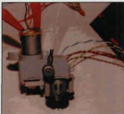
Fig. 7—A simple dynamometer for testing transmissions.
