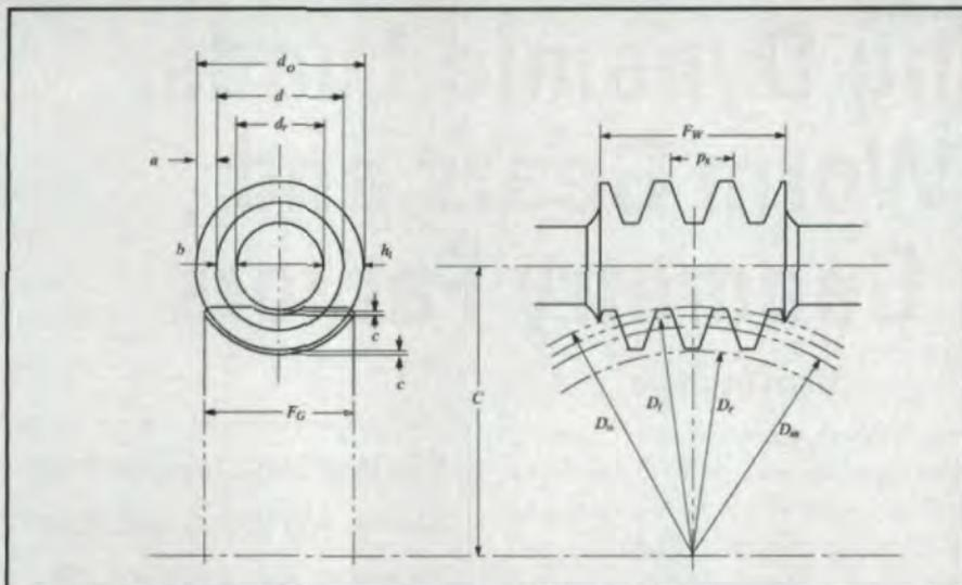
Fig. 1 — Worm gear basic dimensions. Source: ANSI/AGMA 6022-C93.
