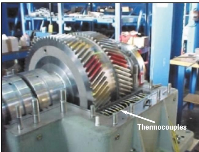
Figure 4—High speed test rig.
