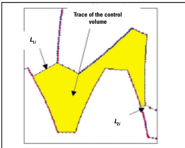
Figure 1—Definition of the control volume and exit flow areas.
