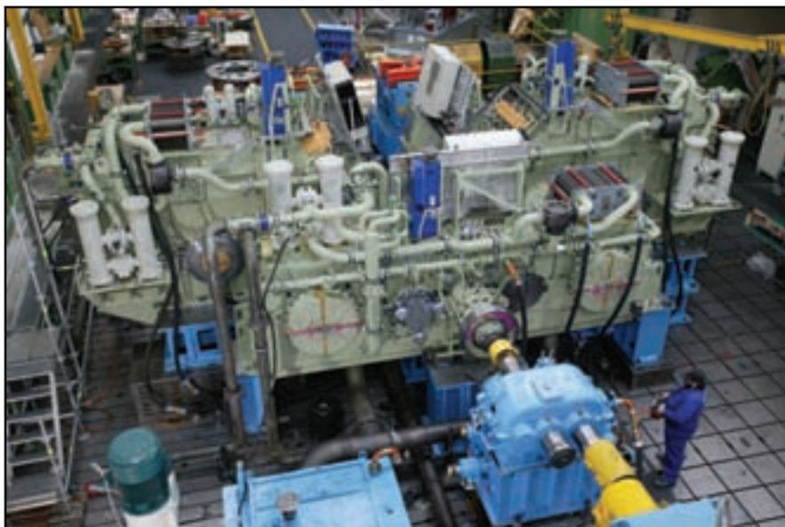
A Complex Gearbox —The combined marine gearbox here, a CODAG, can simultaneously transmit power from a diesel engine and a gas turbine or can transmit power from one or the other separately. Such complicated gearboxes are common among many larger marine vessels. Photo courtesy of Renk AG.
