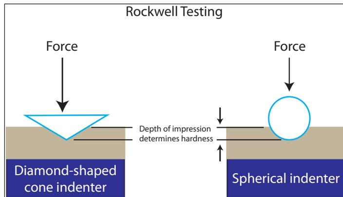
an easier alternative to Brinell testing. It uses a standardized indenter, and the results are largely force independent (although there are special considerations for microindentation tests done at forces of less than 200 g).
