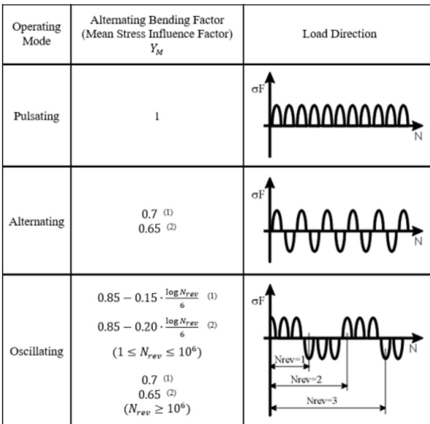
Figure 4 Alternating fatigue according to (Ref. 8) (1) e (Ref. 9) (2).
