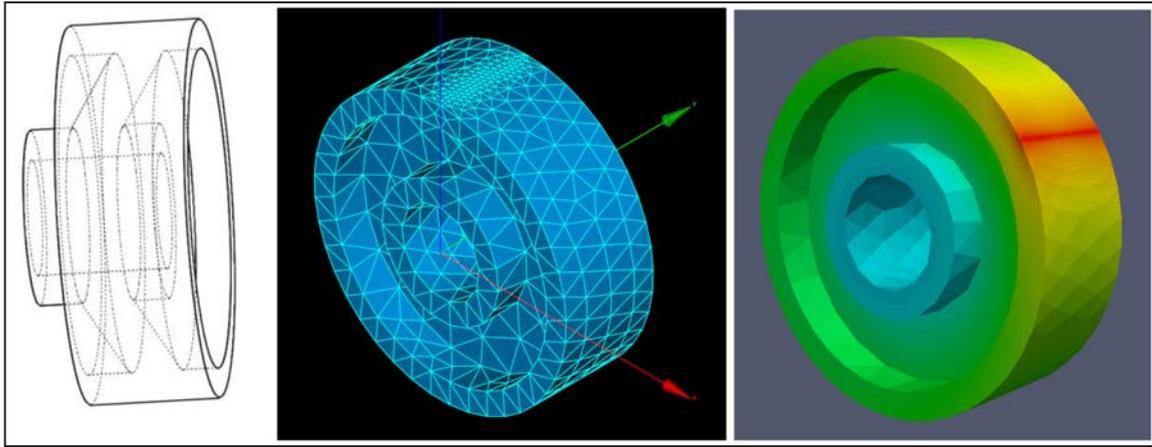
Figure 5 Gear body FEM calculation (Refs. 10 and 15).
