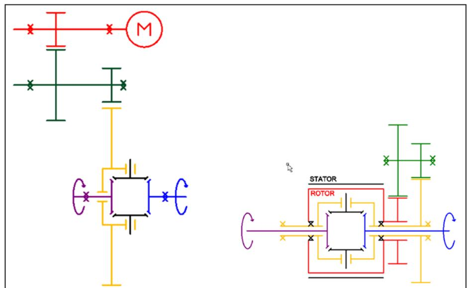
Figure 1 Two different layouts for 2-stage single-speed transmission.
