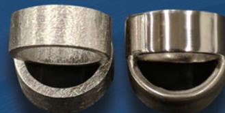
Proprietary coating methods create a smooth cosmetic surface, additional hardness, and corrosion resistance.
