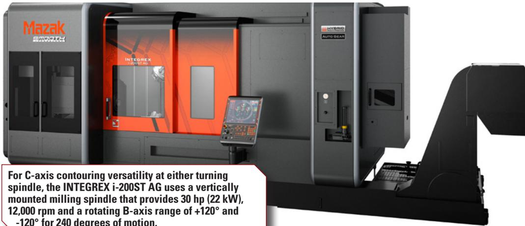
For C-axis contouring versatility at either turning spindle, the INTEGREX i-200ST AG uses a vertically mounted milling spindle that provides 30 hp (22 kW), 12,000 rpm and a rotating B-axis range of +120° and -120° for 240 degrees of motion.
