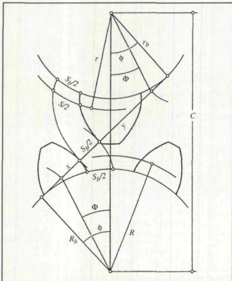
Fig. 2 — Effect of an increase in center distance.
