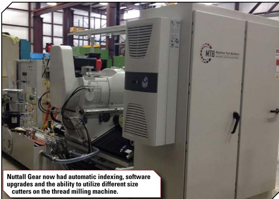
Nuttall Gear now had automatic indexing, software upgrades and the ability to utilize different size cutters on the thread milling machine.
