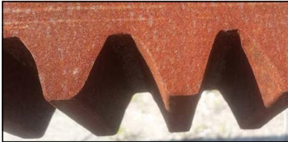
Figure 19 Rack removed from hull.
