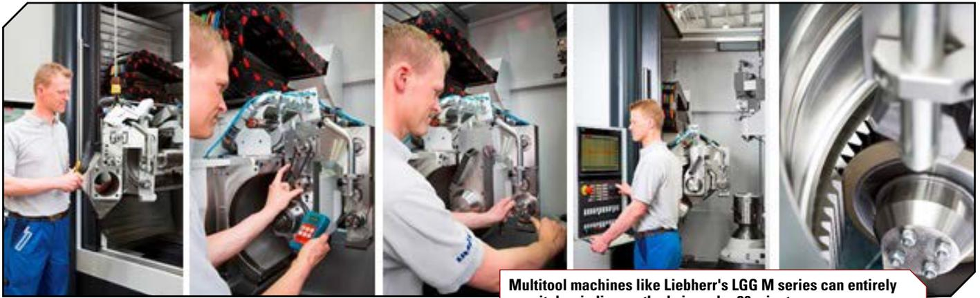
Multitool machines like Liebherr's LGG M series can entirely switch grinding methods in under 30 minutes.
