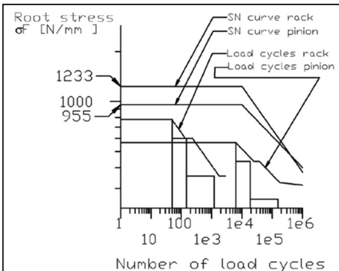
Figure 2 Root bending stress evaluation per ISO 6336.
