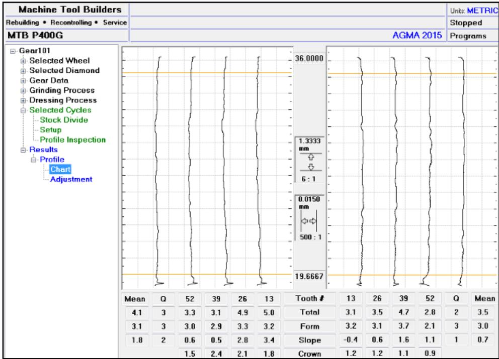
Figure 14 Example of profile inspection and evaluation.
