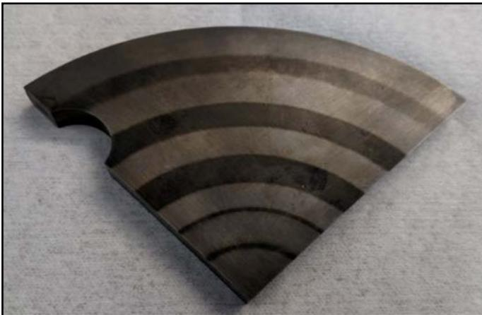
**Figure 5** The standard sample as it appears after a good acid etch.
