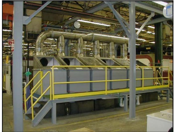
Figure 1 Series of tanks for acid etching in a gear manufacturing facility.
