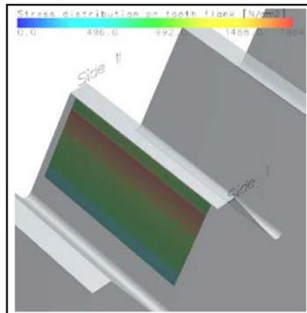
Figure 5 Contact stress for rack.
