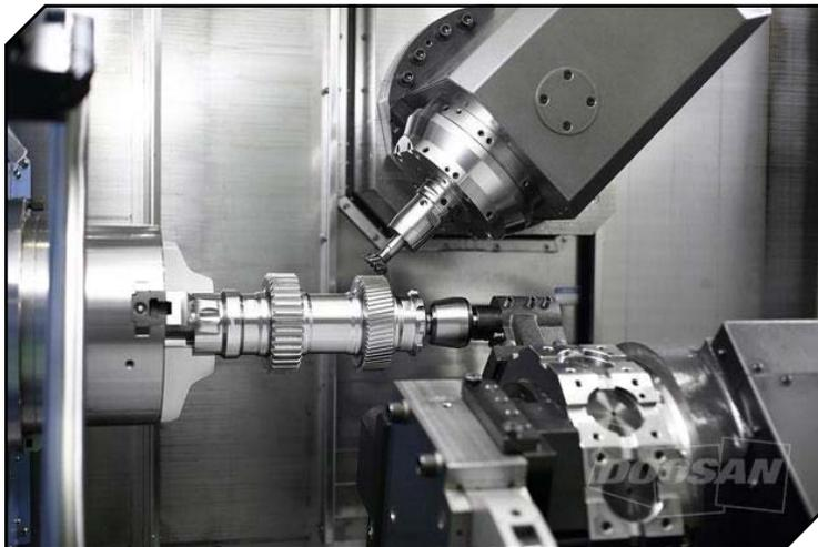
If you want to turn out more completed parts on a single machine with less operator time, Doosan has released the PUMA SMX ST series. These super multi-tasking turning centers have axes everywhere. Both left and right spindles are capable of high accuracy C-axis control and the machine can perform various machining functions like turning, milling and synchronized cutting all with a single set-up.
