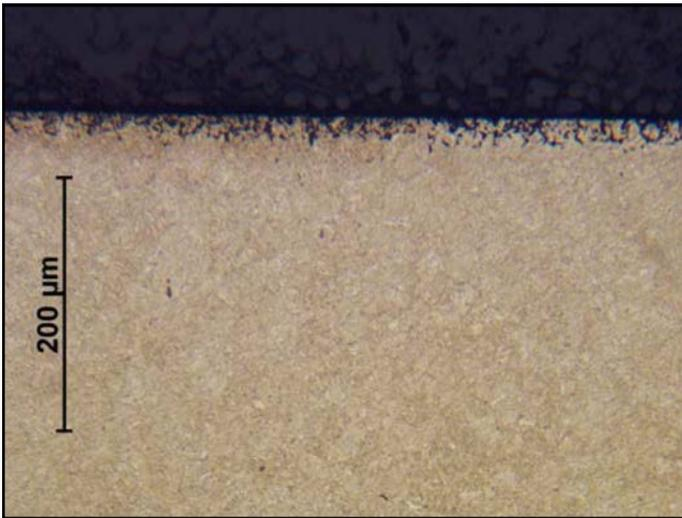
**Figure 4** Non-martensitic transformation products at the surface of the plate after carburize and harden. Removal by grinding is necessary to keep steady temper-back color effects. The grinding must be done carefully so there is no thermal damage.
