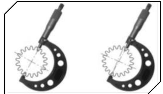
Figure 2 Measurement over balls from AGMA 2002-C16, Figure 10.
