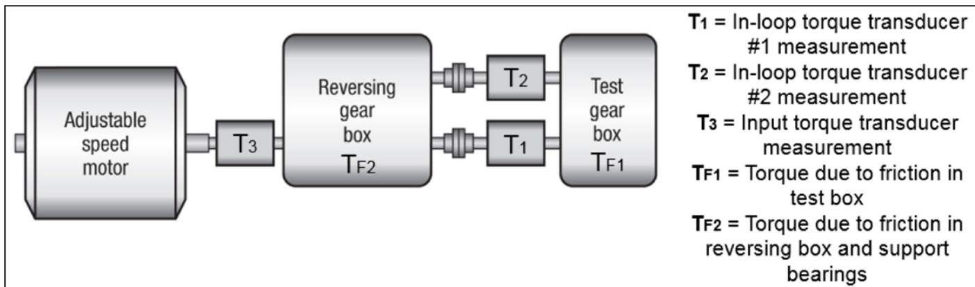
Figure 1 Test rig layout.
