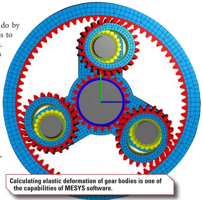
Calculating elastic deformation of gear bodies is one of the capabilities of MESYS software.
