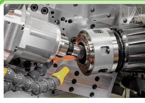
and the C prime axis is equipped with a driven spindle. Vincent Affolter: "This configuration is designed for the power skiving of internal gears. The production of face gears is possible, too."
