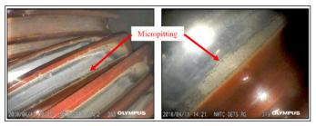
Figure 4—Micropitting on the sun pinion teeth. (Photos by Scott Eatherton, Wind Driven, NREL 61193 and 61194.)
