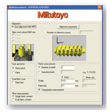
Special CMM software supports measuring different types of worm gears using a touch trigger probe or scanning probe on a CMM.
