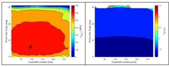
Figure 3—Pressure distribution (left) and specific film thickness (right) across the contact zone for Case 1.
