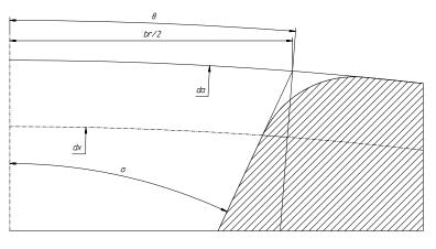
Figure 3—Calculating parameters of pulley profile.
