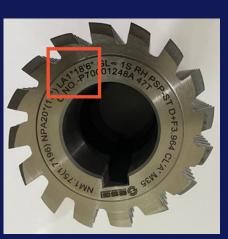
Figure 3—Hob marking for spur gear.
