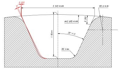
Figure 1—Geometry of a T5 28-tooth pulley.
