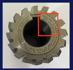
Figure 4—Hob marking for helical gear.
