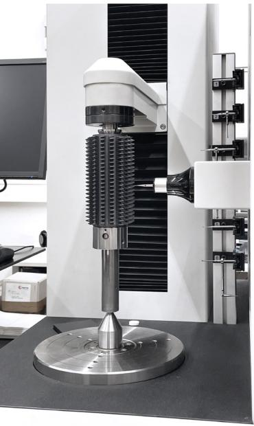
Additionally, the system can be purchased with a dedicated part locator, which allows the operator to position heavier workpieces or dedicated parts more easily in the same, precise, repeatable location each and every time one's loaded.
