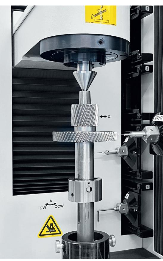
Gleason LeCount Expanding Mandrels seem almost tailor-made for the rigorous demands of today's quality labs. They deliver the extreme accuracies required of high precision workpieces with 2.5 microns (0.0025 mm/0.0001 in.) TIR or better. Their simple design makes it easy for a technician with even minimal experience to ensure a precise, repeatable load/unload of the workpiece in a matter of seconds.
