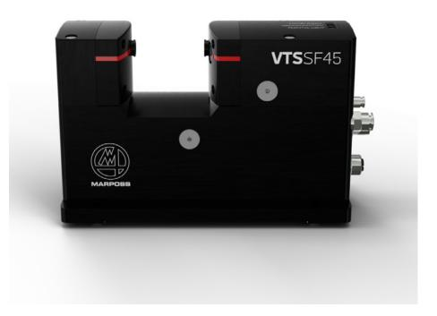
working spaces such as micromachining, semiconductor or moldmaking applications. The VTS SF-45 units are installed inside the machine working area to monitor actual tool working conditions without any contact while the tool can rotate at full spindle speed (up to 80k rpm) during data acquisition. Since there is no need to slow the spindle, presetting time can be reduced and measurement accuracy is increased to better eliminate collision hazards.
