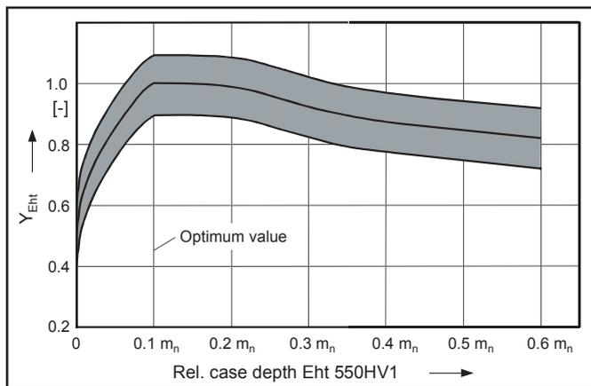
Figure 15—Influence factor  $Y_{Eht}$  for the influence of case depth on tooth root bending (endurance) strength.
