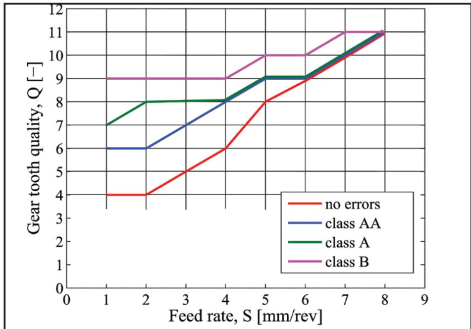
**Figure 9** Gear tooth quality vs. axial feed rate of hob for different hob classes.**Table 6** Gear tooth deviations, results from experiments and simulations
