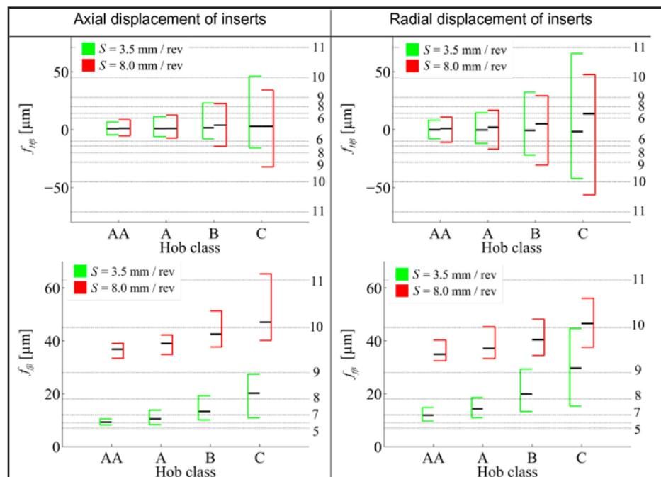
**Figure 7** Result from simulation where the lead deviations are plotted with varying hob classes. On the left ordinate, the gear tooth deviation, and on the right ordinate, the gear quality, is plotted.
