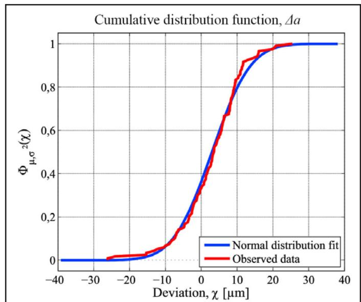
Figure 3 CDF: plot, axial deviation of inserts.
