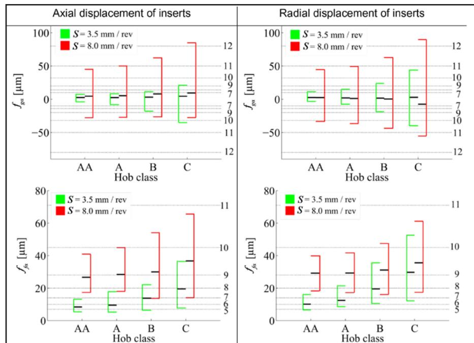
**Figure 6** Result from simulation where the profile deviations are plotted with varying hob classes. On the left ordinate, the gear tooth deviation, and on the right ordinate, the gear quality, is plotted.
