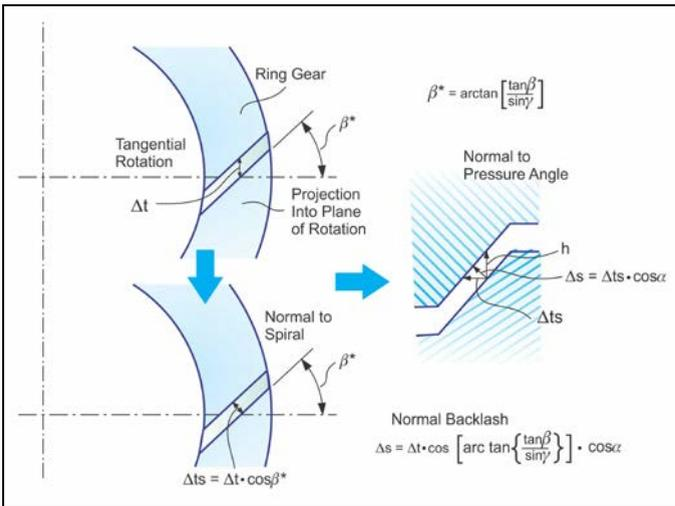
**Figure 2** Calculation of normal backlash  $\Delta s$ .
