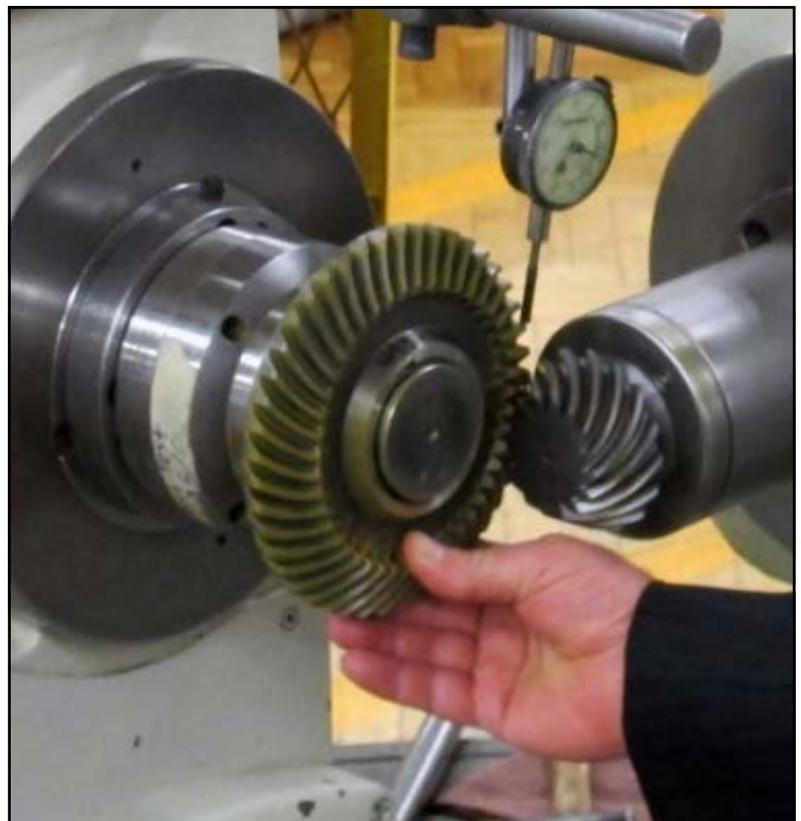
Figure 1 Measurement of normal backlash.
