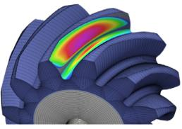
Figure 2—Qualitative distribution of flank pressure and tooth root stress based on FEM influence numbers and influence vectors.
