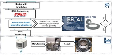
Figure 4—Possible evaluation and manufacturing process.
