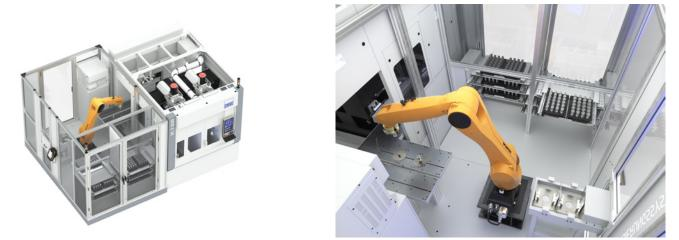
Figure 4—With the drawer system, the workpieces are provided to the robot on different levels. While the drawers are being loaded, the robot in the cell supplies the machine with workpieces.
