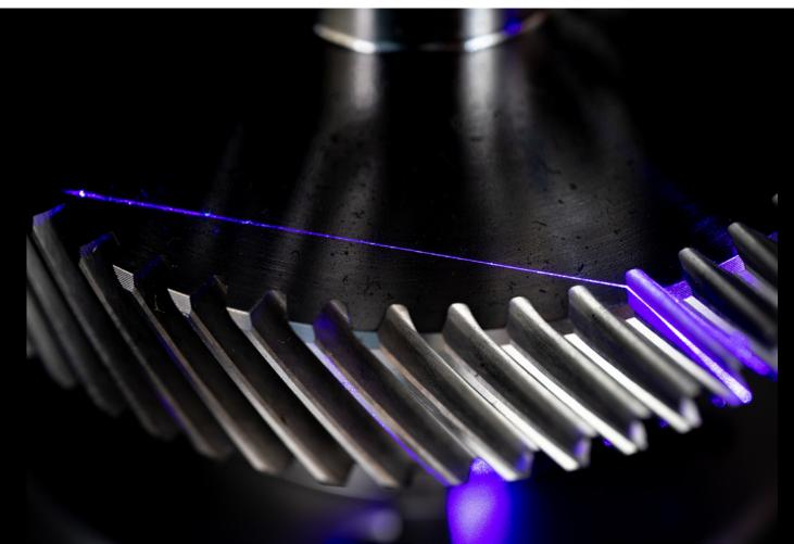
Figure 5—The application of noncontact technology—such as lasers and cameras—is also evolving to tackle the increased need for gear measuring in e-drives.
