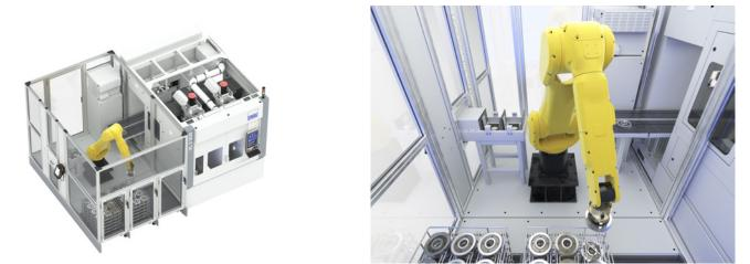
Figure 3—In automation cells with basket stacks, the system is loaded and unloaded by baskets from which the robot picks up or deposits the oriented workpieces. The empty baskets are transferred to the stack by the robot.
