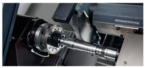
Figure 12—Grinding in single clamping with WMZ Spindle Technology. (Source: BUDERUS Schleiftechnik)
