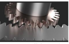
Figure 4—Animation of the skiving process. (Source: Pittler T&S)
