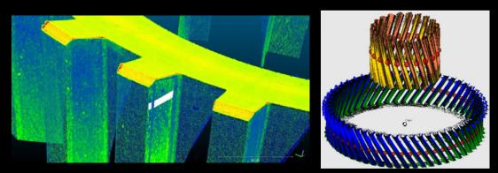
Figure 6—In Marposs' newest system laser profile sensors and the optical triangulation principle help reconstruct a 3D model of the component being measured.
