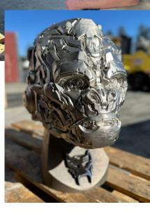
parts. The part is shown as printed so you can see the final texture, but the base features portions that have been machine polished, like how parts would be finished after being printed.
