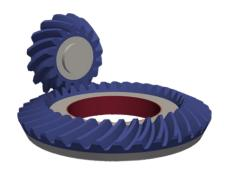
Figure 3—Example BECAL-representation of bevel gear set.
