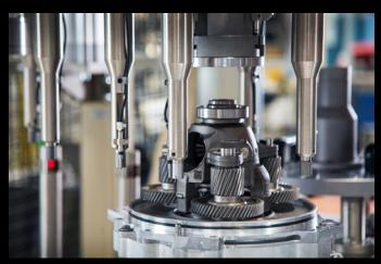
Figure 1—Gears for electric drives need to be designed with tighter manufacturing tolerances, especially around profile and lead features.
