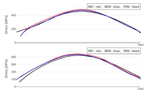
*Figure* 5—2D *Tooth root stress distribution.*
