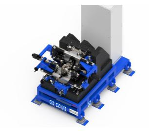
Figure 2—This gear tester from Marposs works on the single flank testing method where a master gear meshes with the component under inspection, identifying defects not detectable with traditional production tests.
