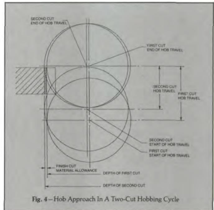
Fig. 4—Hob Approach In A Two-Cut Hobbing Cycle
