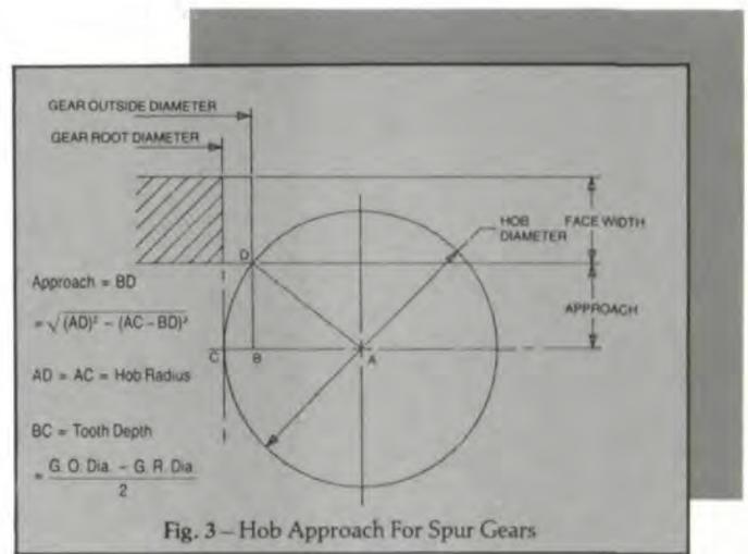
Fig. 3—Hob Approach For Spur Gears
