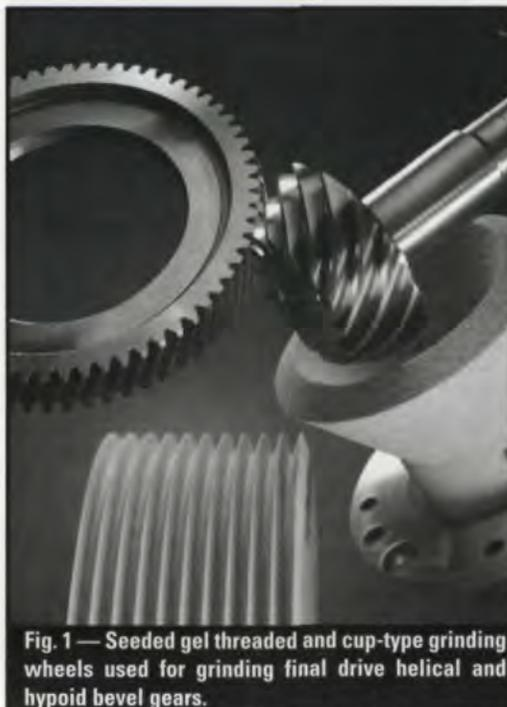
**Fig. 1 — Seeded gel threaded and cup-type grinding wheels used for grinding final drive helical and hypoid bevel gears.**
