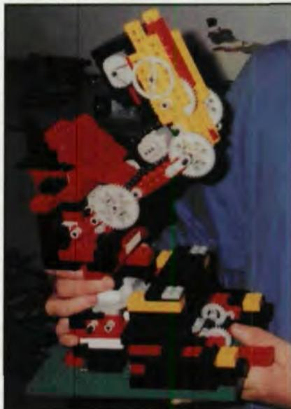
and 40 teeth. And very important to junior transmission designers, Lego parts are manufactured to a tolerance of  $\pm .005$  mm.
