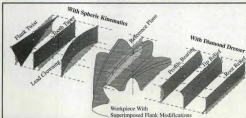
Fig. 4 — Flank modifications with spheric honing.
