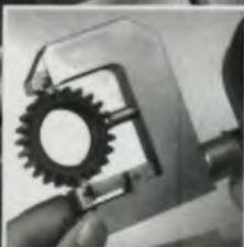
Built-in gage pins save time and eliminate the possibility of operator variability.
