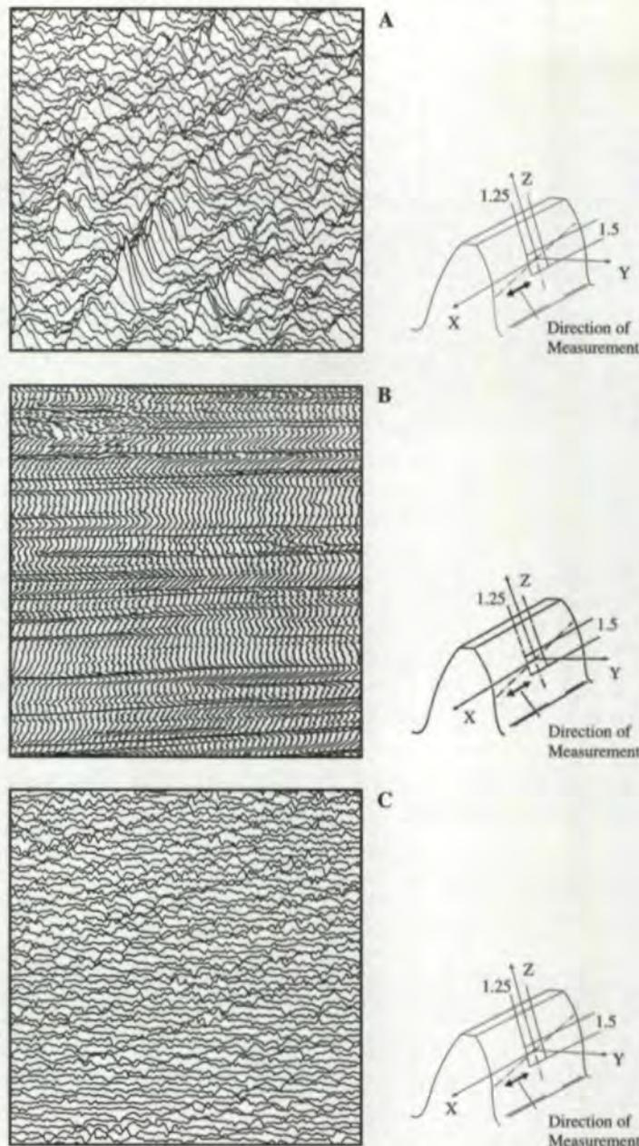
Fig. 2 — A) Surface structure of a shaved flank. B) Surface structure of a ground flank. C) Surface structure of a honed flank.
