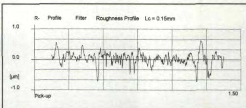
Fig. 3 — The roughness profile is the signal after filtering with a cutoff of .15 mm. Note that the amplification of this chart is 25 times greater than that of the unfiltered profile. Also, the profile is centered down the middle of the chart and shows no residual curvature, indicating that the cutoff was small enough to remove any residual curvature from the unfiltered profile.
