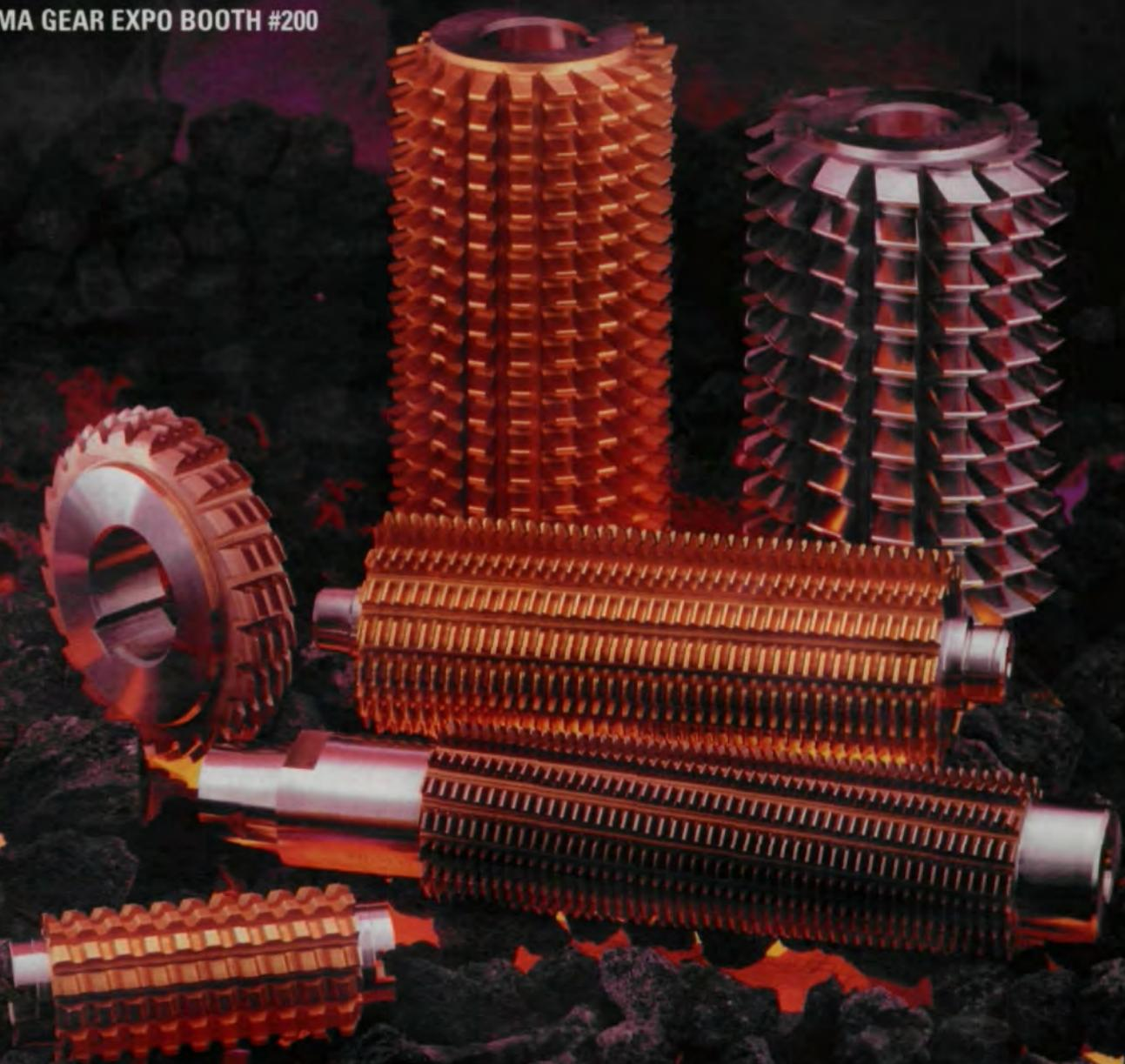
The only way to get top quality gears, is to machine them with precision hobs. At Star Cutter, we utilize the most advanced technology available to insure that each of our precision hobs will deliver the exact performance you need — cut after cut, day after day.
