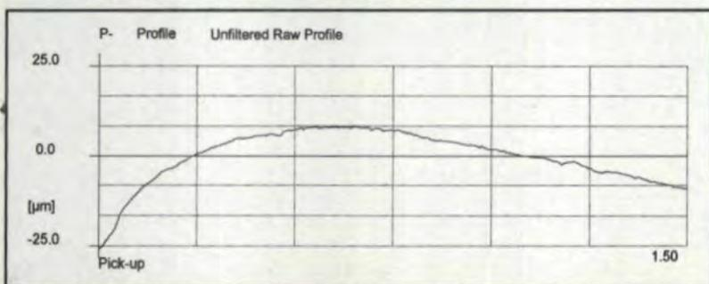
Fig. 2 — The unfiltered profile generated by the signal from the pickup shows the significant amount of curvature that results from the interaction of the skid and the involute form. Also, the roughness signal is hardly discernible.
