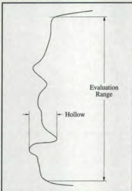
Fig. 11 — "Hollow" is the reversal of curvature.
