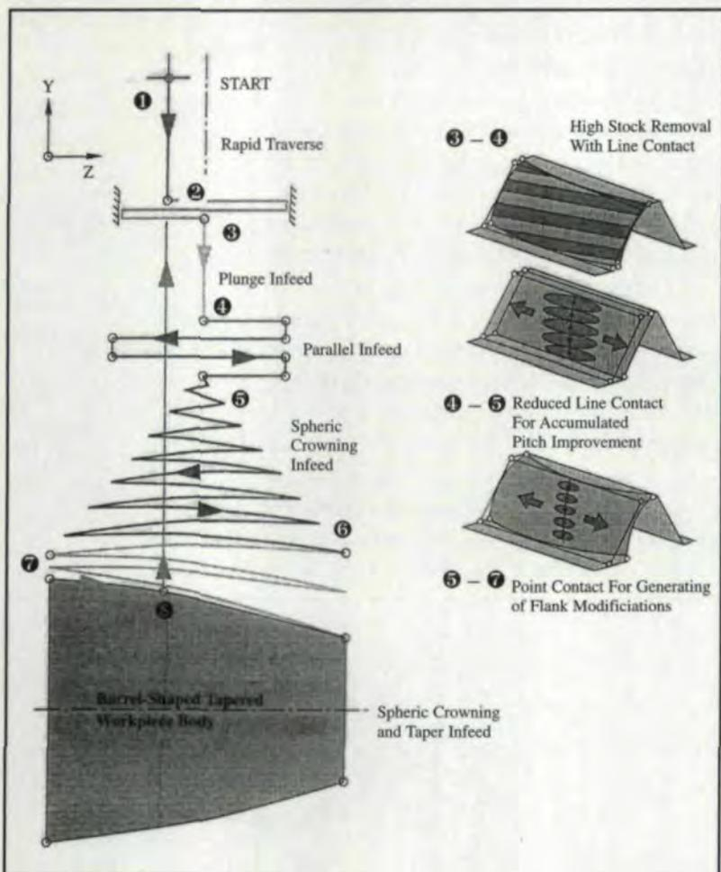
Fig. 7 — Tooth contact behavior between tool and workpiece.
