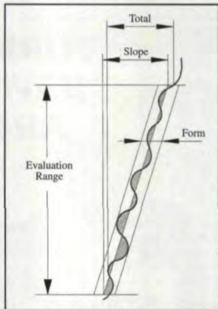
Fig. 7 — Total, slope and form errors.
