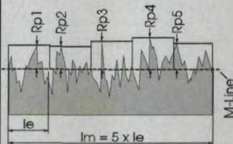
**Pc - Peak count:** A peak count taken over a standard length of 10 mm of the filtered roughness profile. Whereby a peak is only read after the profile has passed through both a lower and an upper variable preset threshold  $C_1$  and  $C_2$ . Both threshold lines are set parallel to the 'center-line'.
