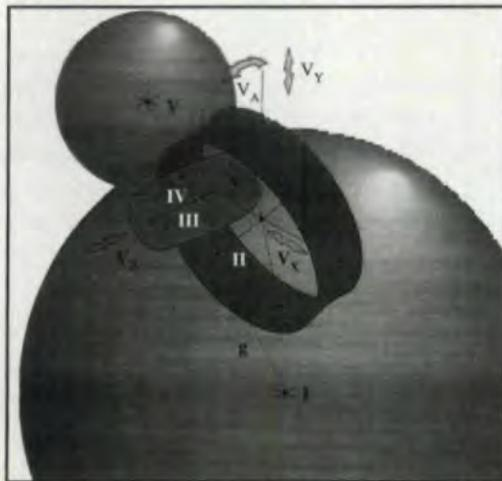
Fig. 3 — Basic kinematics of the spheric honing process.
