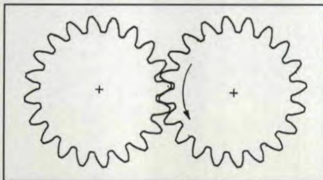
Fig. 1 — Gear wheels with asymmetrical tooth profiles.
