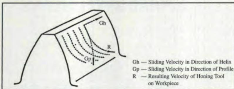
Fig. 1 — Kinematics of machining.
