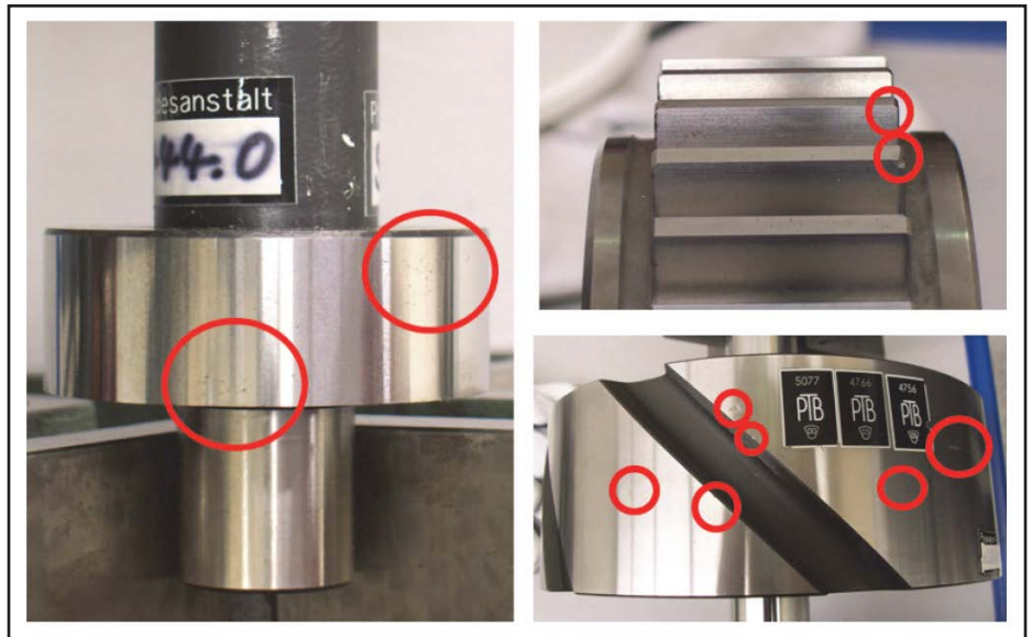
Figure 4 Damages inflicted on the measurement standards surface.
