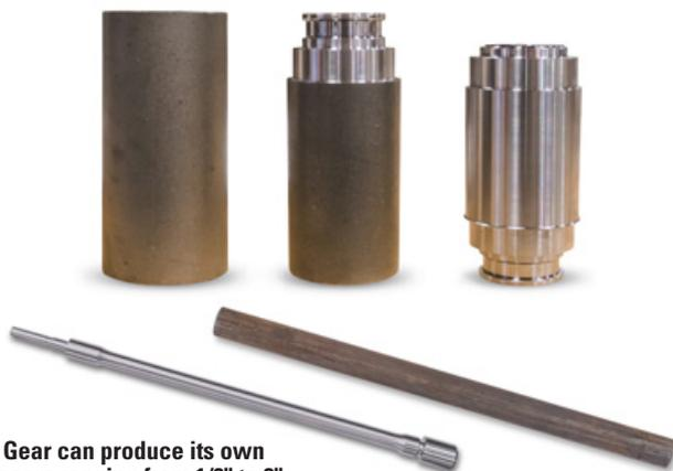
Forest City Gear can produce its own blanks for gears ranging from 1/8" to 8" in diameter, shafts up to 16" long – in lot sizes from one to a thousand.
