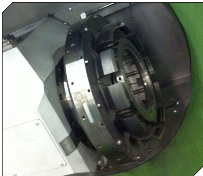
Ringspann clamping fixture for gear skiving.
