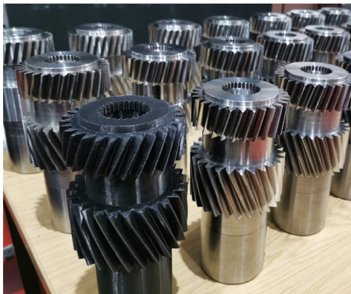
Figure 7 Gear Shaft B component geometry (Spline A internal, Gear B bottom external, Gear C top external).
