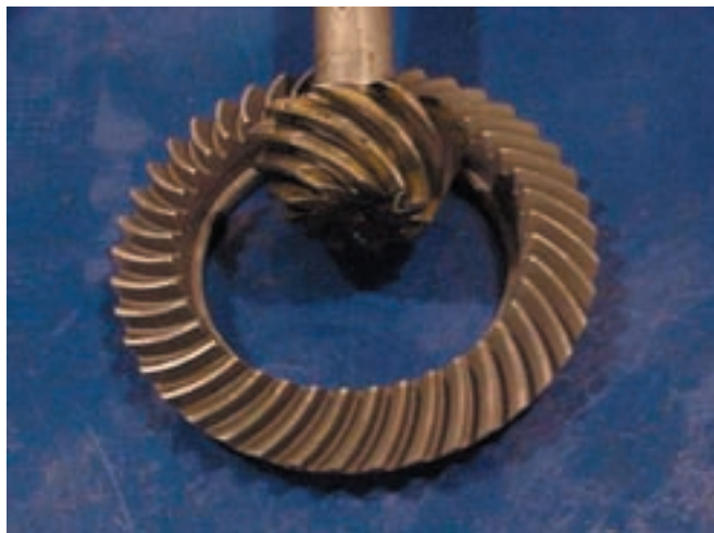
Figure 11—Gear set photo before superfinishing process.
