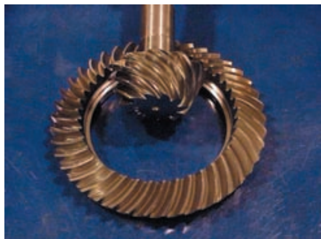
Figure 12—Gear set photo after superfinishing process.
