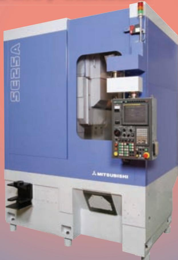
Each of our E series machines have been designed for a specific application. Using the tools of Finite Element Analysis and three dimensional CAD, we have been able to optimize our machine designs to efficiently and economically produce gears. Each unique design is capable of handling all of the varied loads, stresses, heat and process byproducts generated by the cutting or grinding conditions.
