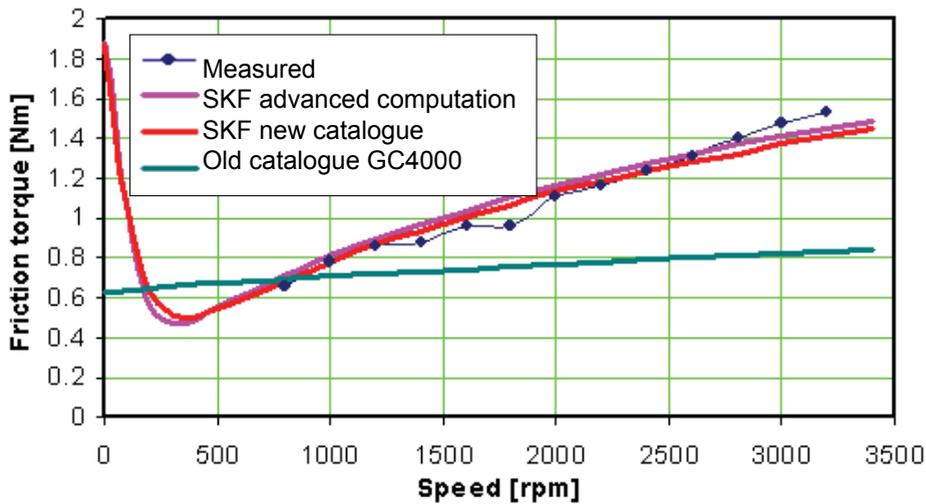
Figure 4 Model prediction and measurement—tapered roller bearing.
