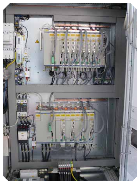
All machine axes are driven by NUMDrive C servos, controlled by a NUM Flexium CNC system.
