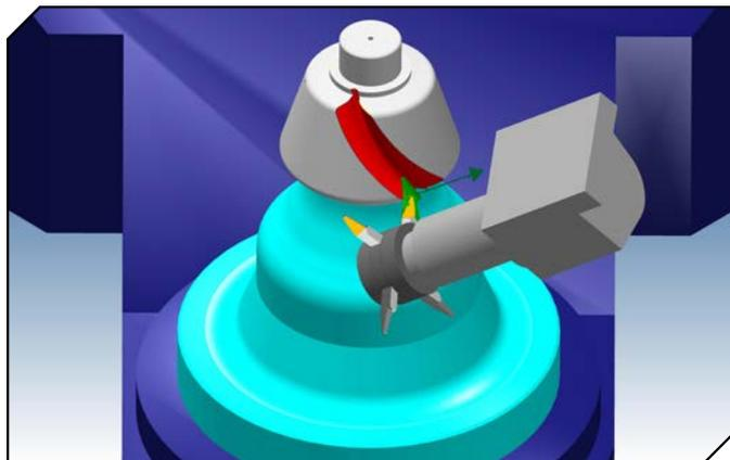
Figure 2 3D view of all components involved in the deburring task.
