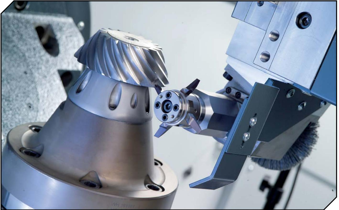
**Deburring or chamfering of gear teeth is gaining attention in practical settings.** And with a view to make the production sequence as efficient as possible, it is becoming increasingly important to be able to implement the deburring tasks directly on the cutting machine after spiral cutting. Read on to find out how complex this seemingly simple task can turn out to be, and how a new deburring concept provides for enhanced efficiency.
