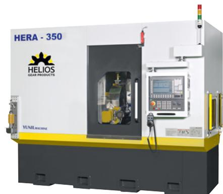
gears and splines. It also features a high-swivel head for worm and thread milling. Manufacturers of parts up to 90 mm (3.543 in) diameter and 3 module (8.5 DP) should visit the Helios booth to see the machine in action.
