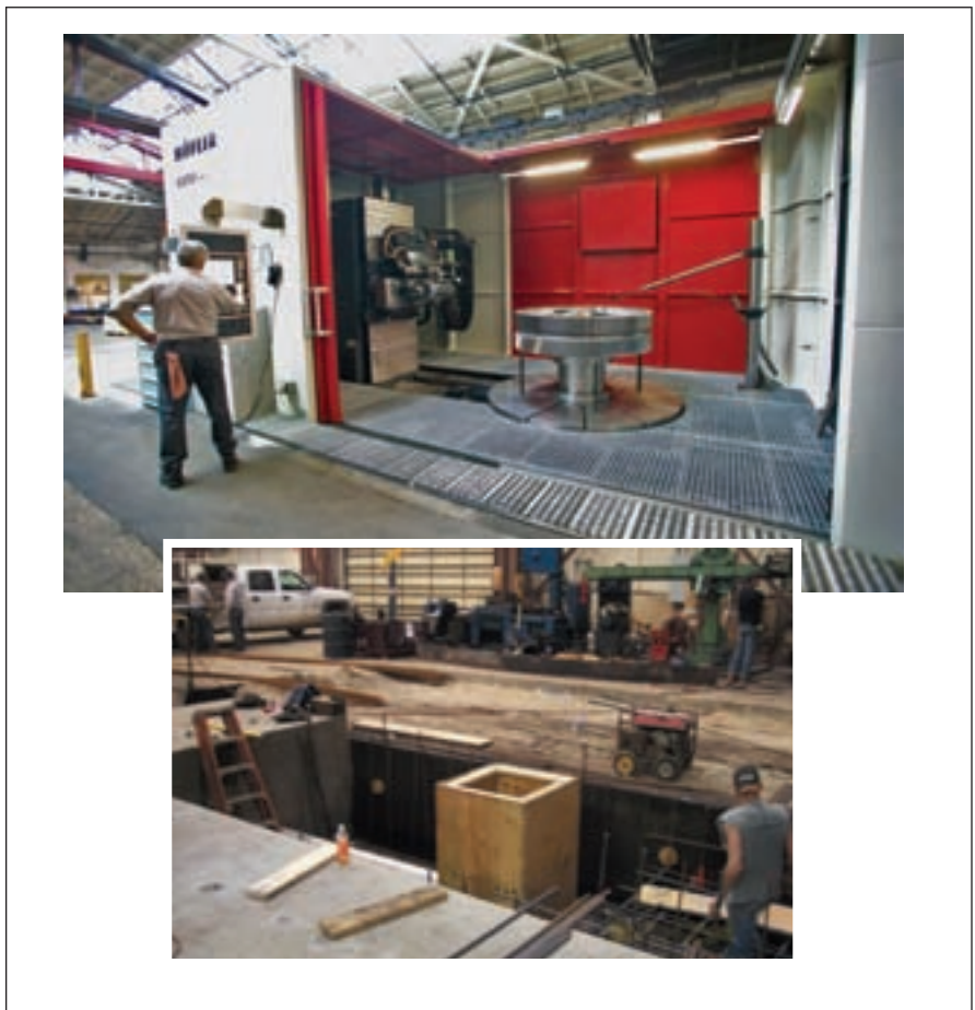
(Top photo) Big gears and those who make them will continue to be a mainstay in 2009. (Courtesy Brad Foote Gear Works.) (Bottom photo) HMC personnel preparing the way for the Hoffer 600 form grinder, the world’s largest gear grinder. (Courtesy HMC.)
